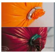
Flat Clips are recommended for sensitive packagingmaterials, such as natural sausage casings. The rounded and brush-finished ends of the clip close softly without doing any harm to the material.
