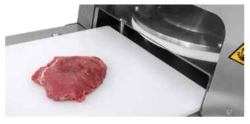
The MAGA® Meat Press automatically starts the flattening process when the tray is inserted.
